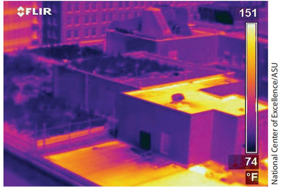
Temperature differences between a green and conventional Roof; green roof measures almost 80degF (40degF) cooler than the neighboring conventional roof
